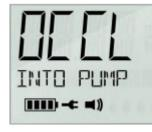
If the display shows OCCL INTO PUMP and an audio alarm sounds, the feed cannot be delivered due to a blockage between the feed container and the pump
